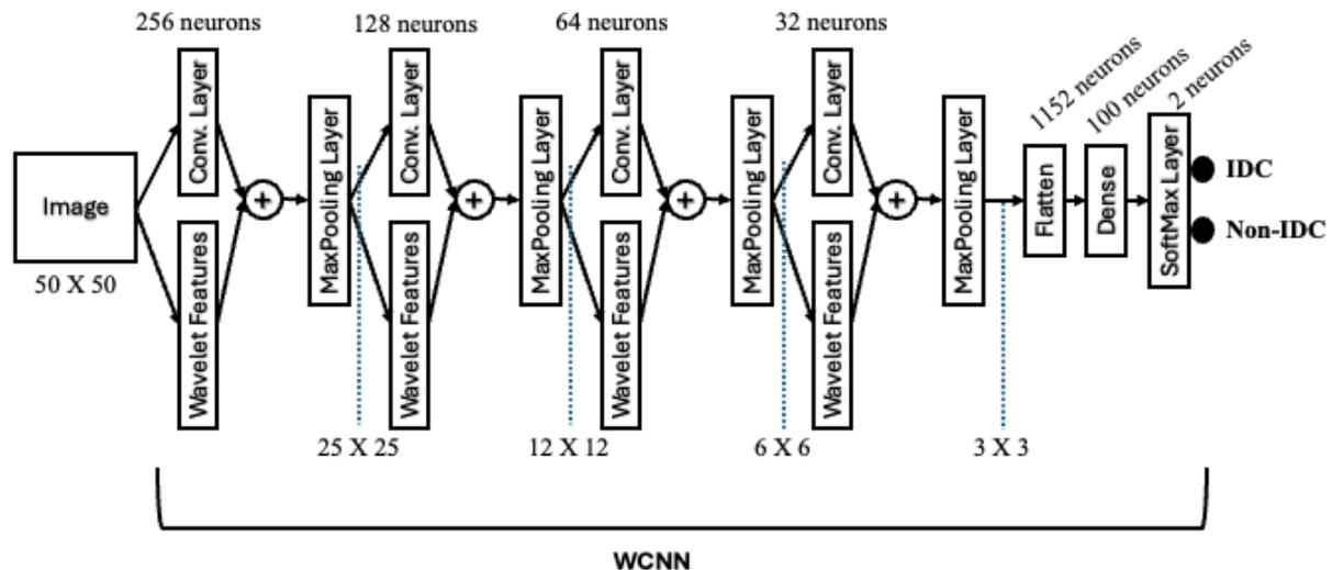
**Figure 3.** Architecture of the proposed WCNN model
